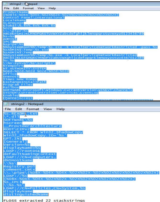
Figure 8. Identifying ASCII and Unicode Strings using STRINGS and FLOSS
