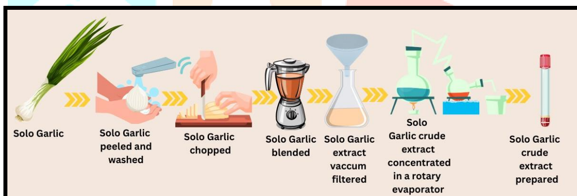
Fig. 2. Schematic illustration describing steps involved in preparation of aqueous crude extract of Himalayan Solo Garlic.
