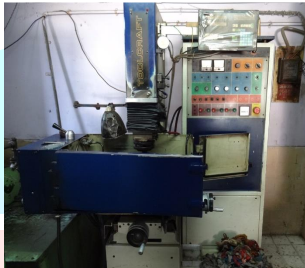
Fig. 1 Electrical Discharge Machine used for performing experiments
