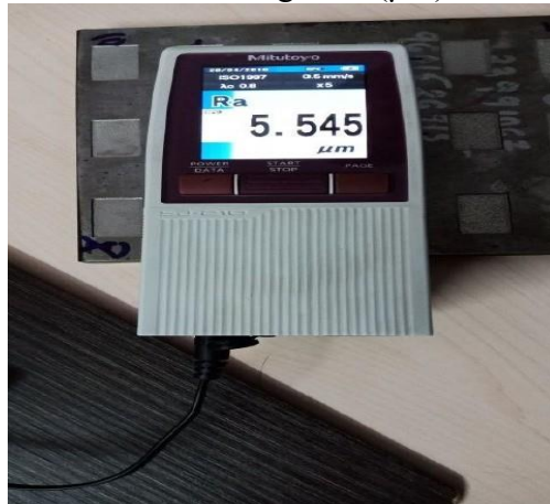
Fig. 4 Mitutoyo SJ 210 Surface Roughness Tester
