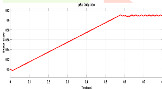
Fig.21 Simulation result of Duty ratio of zeta converter (P&O)
