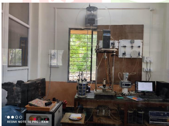
FIGURE 1: CYCLIC TRIAXIAL TESTING MACHINE SETUP
