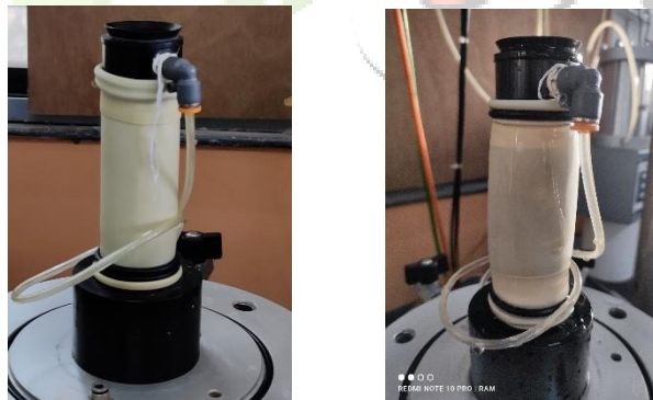
Figure 4 : Sample before Liquefaction & Sample after Liquefaction
