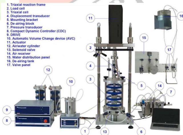
FIGURE 2: PARTS OF CYCLIC TRIAXIAL TESTING MACHINE
