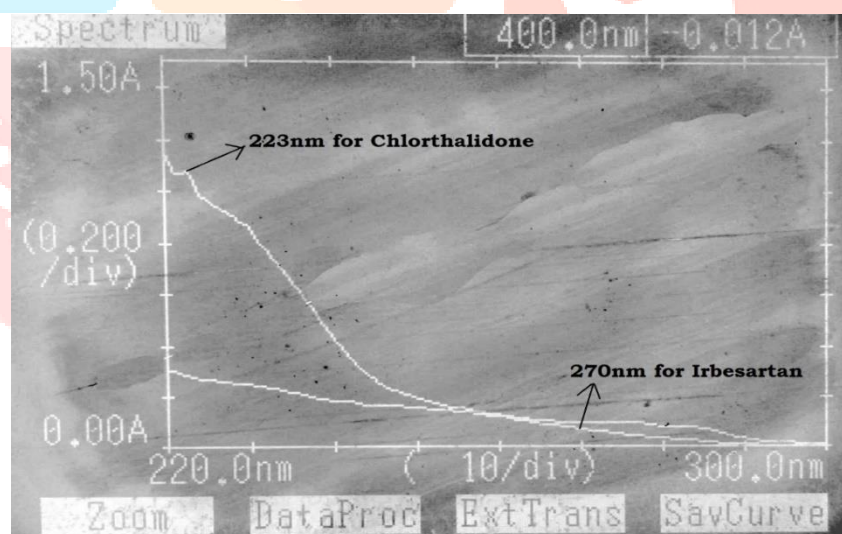
Figure 1: Zero order overlain spectra of 10 \mu\text{g/ml} of IRB and CHL respectively
