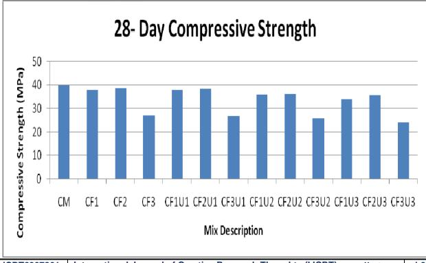
**Discussion on Compressive Test:** The results of the compressive strength test showed that the conventional concrete had a strength of 27 MPa after 7 days and 40 MPa after 28 days. The addition of fly ash had a negligible effect on the strength of the concrete. However, when fly ash was used in combination with waste engine oil, the compressive strength values decreased progressively with an increase in the percentage of fly ash and waste engine oil.
