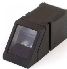
Fig.3.2: R307 Finger print Sensor
