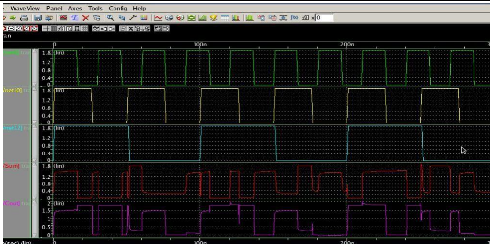
Fig 2: Output Waveform of Conventional 10T 3-2 and 4-2 Adder
