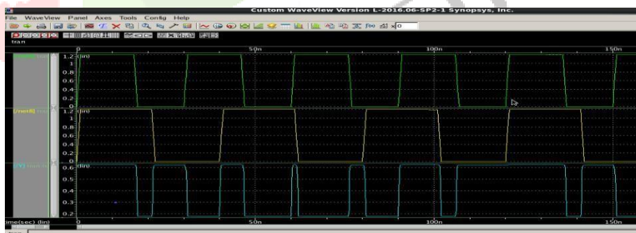
Fig 1: Output Waveform of proposed 3T XNOR Gate
