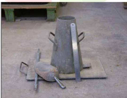
Fig 2 Slump Cone Test
