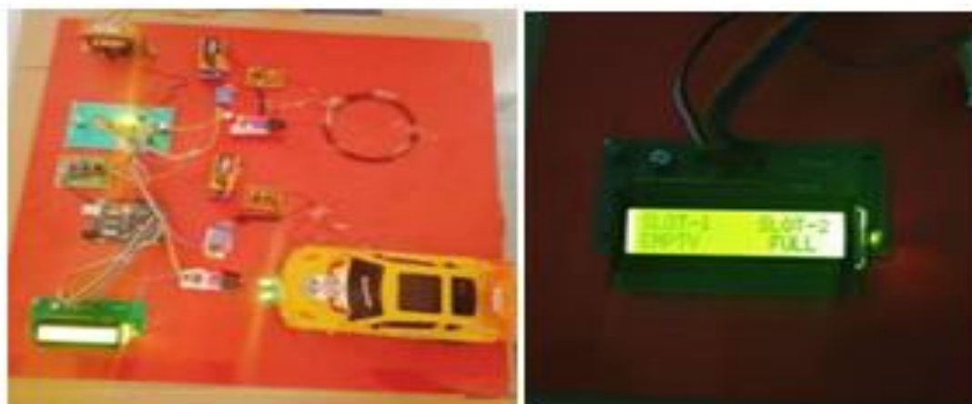
Fig7: LCD displays output as slot2 is full
