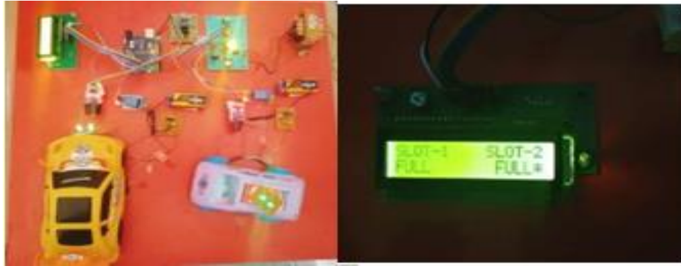
Fig8: LCD displays output both slots are full
