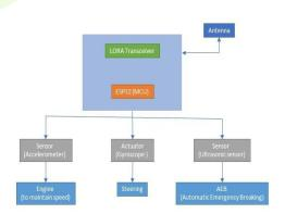
To receive data, the ESP32 can configure the LoRa transceiver to listen for incoming messages and notify the ESP32 when a message is received. The ESP32 can then process the received message and take appropriate action, such as sending a response or triggering an event.
