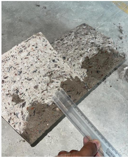
Water permeability test
