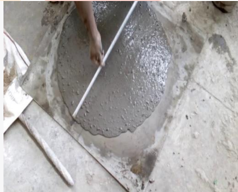
Slump flow test
