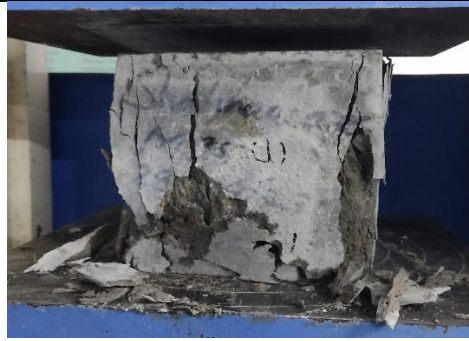
Fig. 2.3. Compressive strength test
