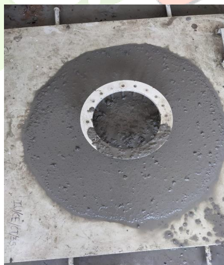
Figure 3 J Ring test
