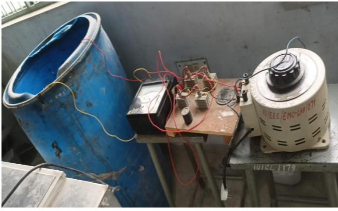
Fig 1. Set up of accelerated corrosion regime.
