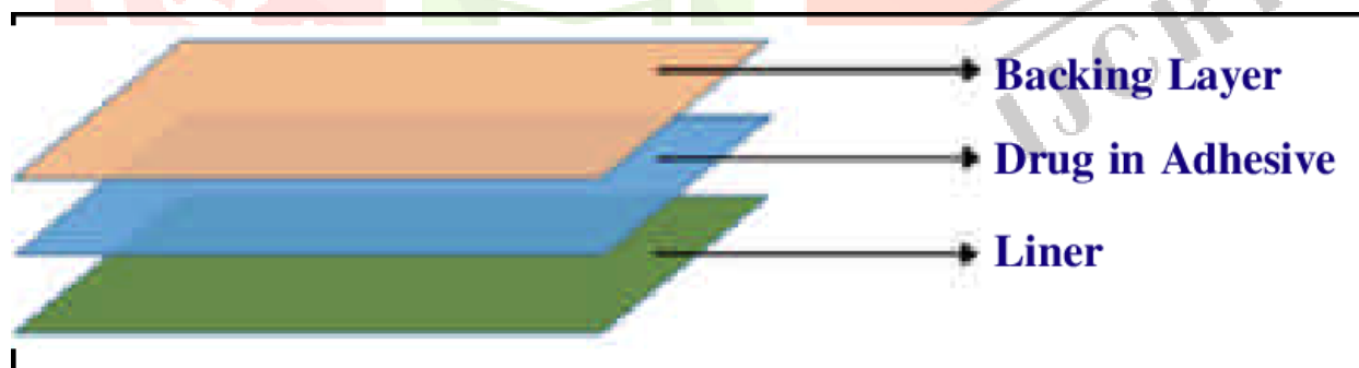
Figure 2: Single layer drug-in-Adhesive
