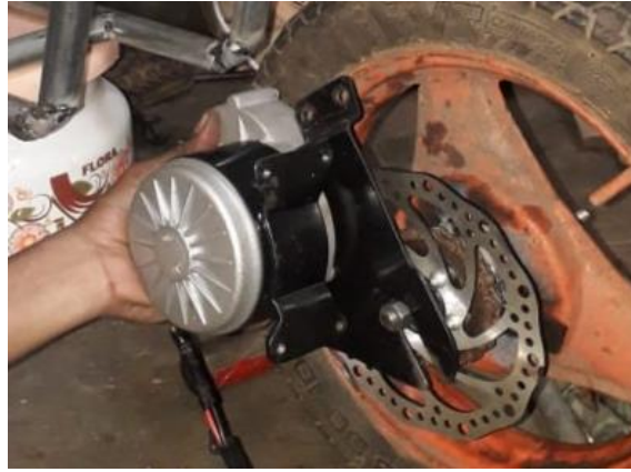
Fig.4.2 24 V and 250 W standard DC motor
