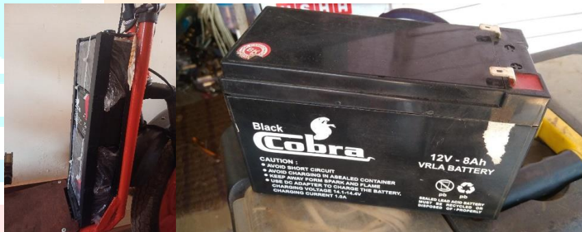
Fig.4.3 12V 8 Ah battery pack
