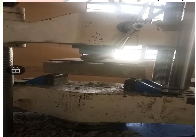
Fig. 1 - Flexural test on Specimens
