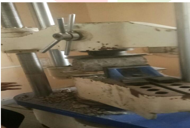
Figure No 2: Split tensile Test on Geopolymer Concrete
