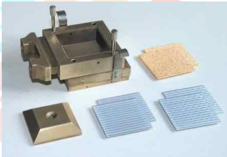
Fig 14: Shear Box, Porous Stones, Grid Plates, Loading pad
