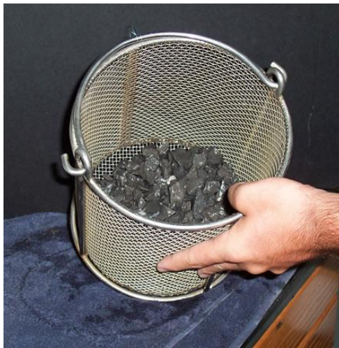
Figure 3.10 Specific gravity test
