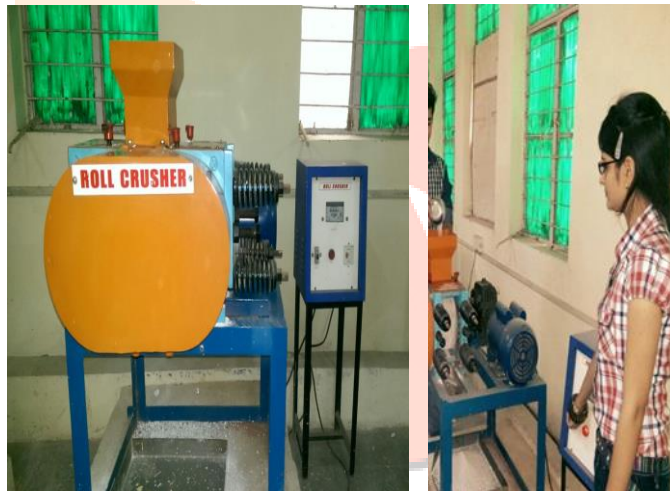
Figure 3.13 Crushing lime using roll crusher
