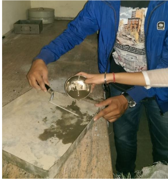
Figure 3.5 Consistency of cement test
