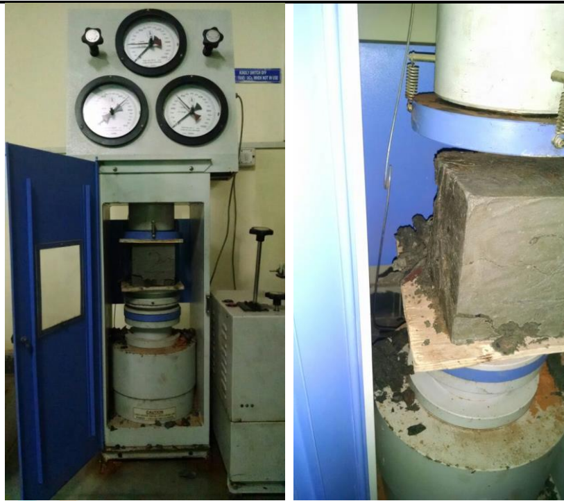
Figure 3.12 Block's compressive strength testing machine
