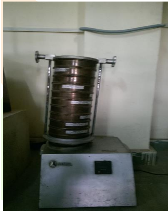
Figure 3.4 Sieve analysis of fine aggregates
