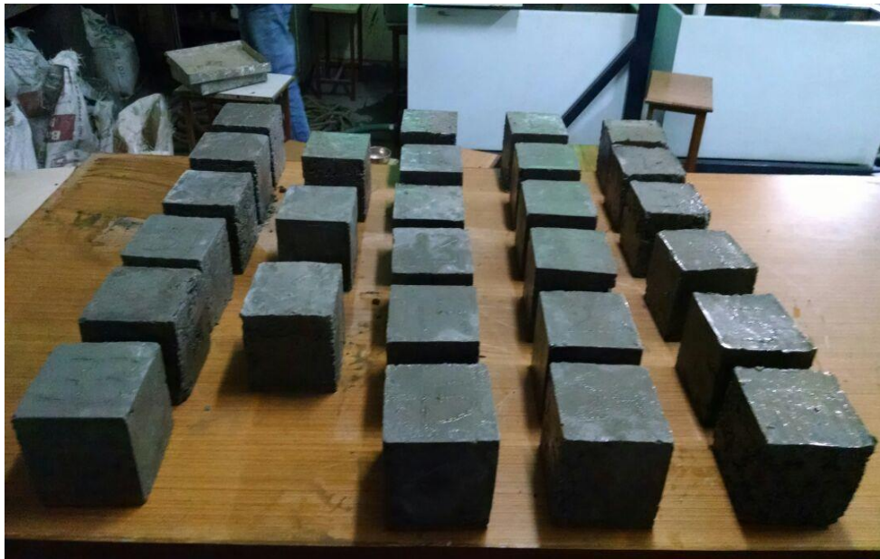
Figure 4.2: Casted concrete blocks
