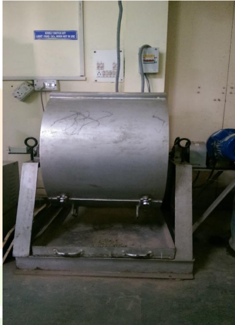
Figure 3.1 Los Angeles abrasion value test
