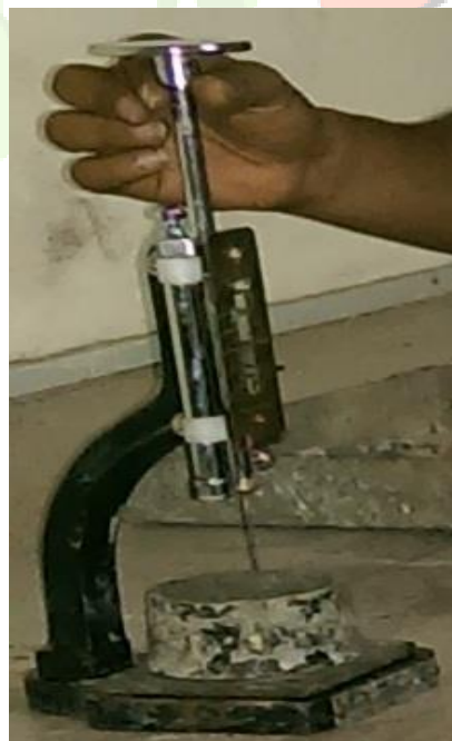
Figure 3.6 Initial & final setting time test
