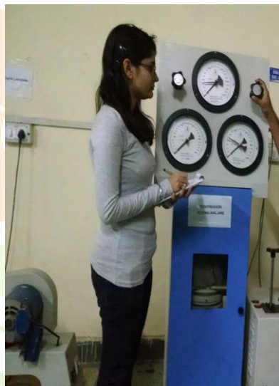
Figure 4.3: Compression testing of blocks
