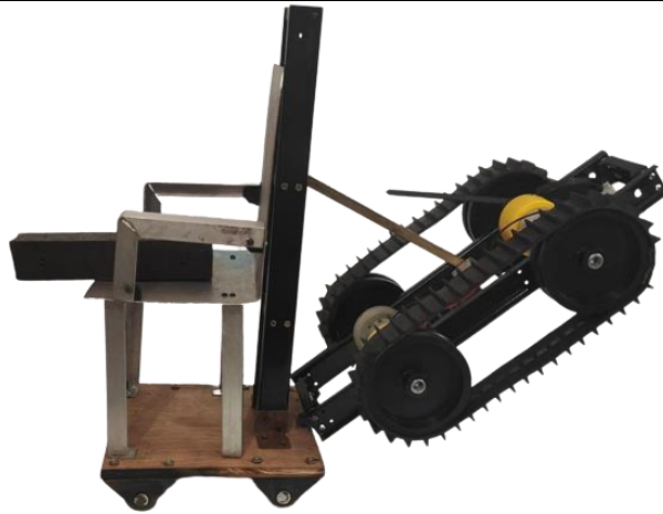
Fig. 3.3: Fully fabricated mobile stair lift
