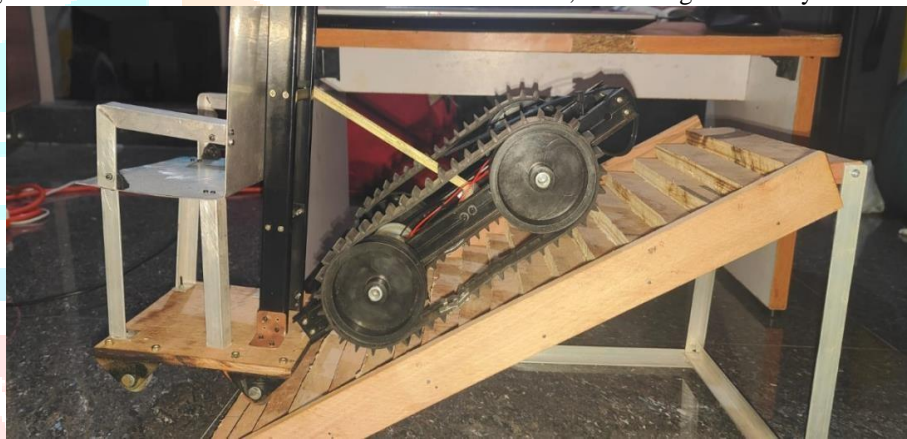
Fig. 3.4: Wheelchair climbing the stairs
