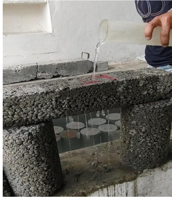
Fig.2 Water passing through porous beam
