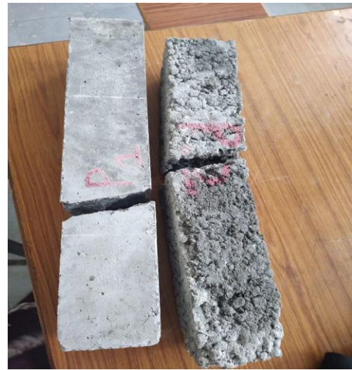
Fig.6 Failure of beams
