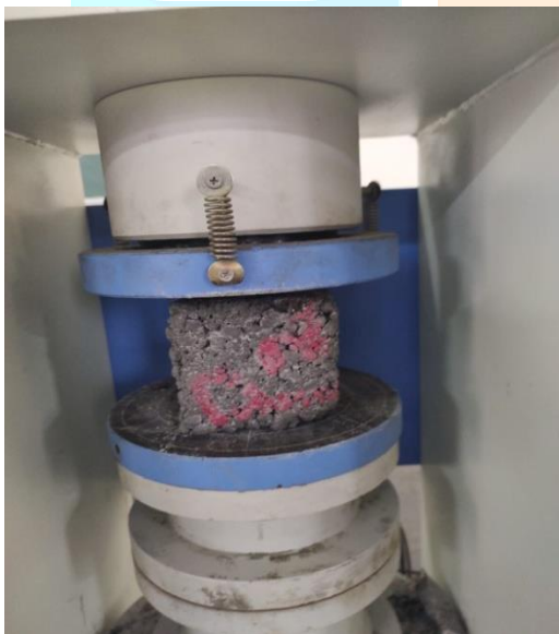
Fig.3 Porous cube under compression
