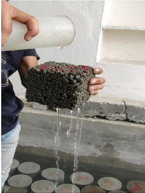
Fig.1 Water passing through porous cube
