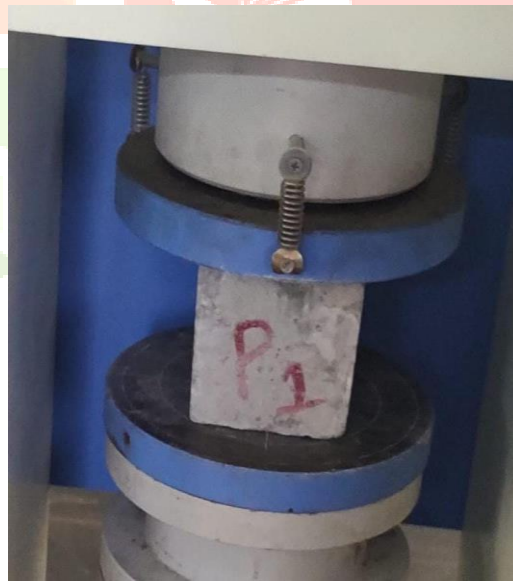
Fig.4 Conventional cube under compression
