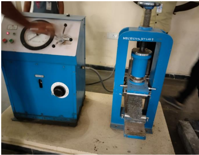
Fig.5 Beam under flexural strength test
