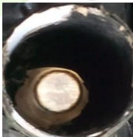
Installing a 70mm focuser above the secondary mirror
