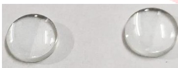
Plano Convex 20mm diameter and focal length 47mm length 15mm
