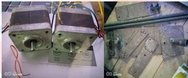
nema 17 stepper motor 4.8 kg-cm mechanical part for mount
