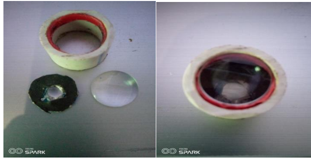
Eyepiece 15mm focus length
