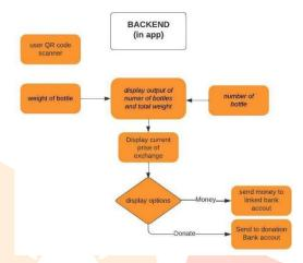
When the user scans the QR code once it has been presented, the machine dispenses the bottle and measures its weight and sends rewards accordingly to the mobile application which can further be redeemed for physical money.
