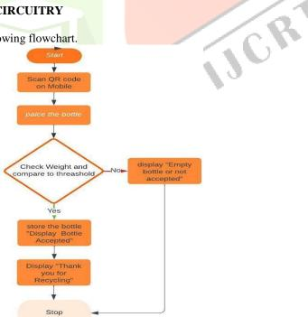
The bottle may be put into the chamber once the user scans the displayed QR code. If the bottle weighs less than the predetermined amount, it is taken inside the chamber and the message "BOTTLE ACCEPTED" is shown. The word "THANK YOU" is displayed to show how much are appreciated for their contribution to the recycling process. The bottles are rejected and labelled "EMPTY BOTTLE" if the weight of the bottle measured is more than the pre-set value.
