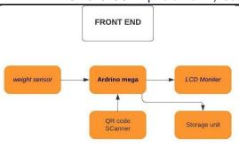
The front end of the process uses an Arduino Mega that is programmed to show the weight of the bottles gathered. The sensors attached to the Arduino Mega are used to measure weight, and the LCD is used to show the information.
