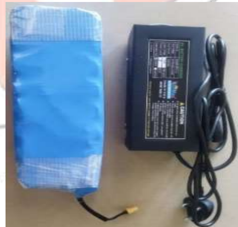
Fig 5 – Battery and charger set
