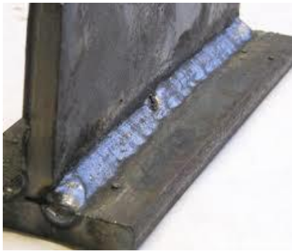
Figure 2 Transverse fillet weld joint
