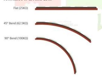
When the sensor is bent, the conductive layer is stretched, resulting in a reduced cross section (imagine stretching a rubber band) and increased resistance. At a 90° angle, this resistance is approximately 100K.
