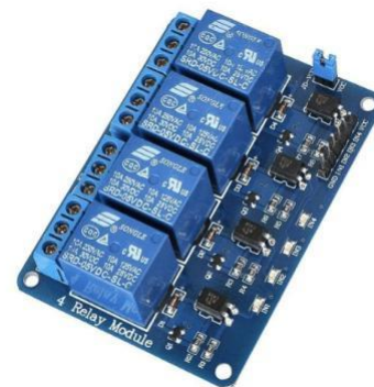
Fig. 2. Four channel relay module
