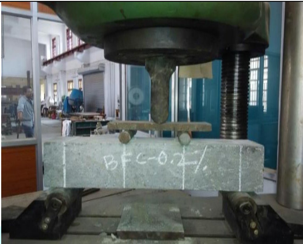
Fig. 3.5.1 Loading Arrangement for Load-Displacement Test
