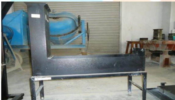
Fig. 3.2.3.3 L-Box Apparatus & Schematic Diagram
