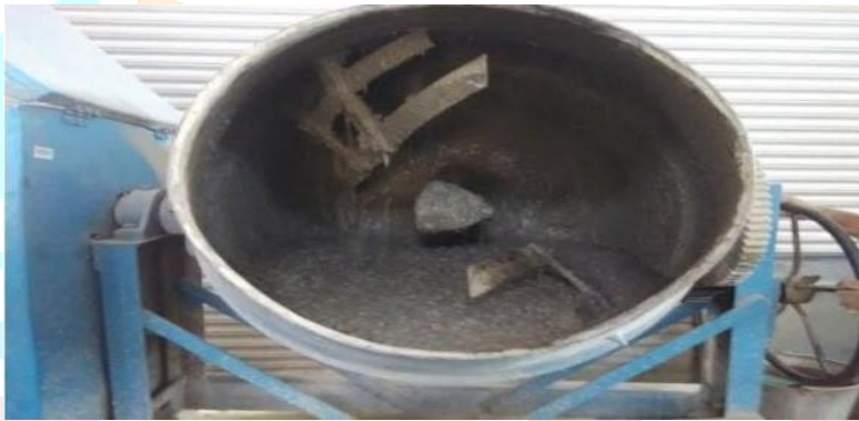
Fig.3.2.1 Concrete Mixture Machine & Preparation of SCC Mix
