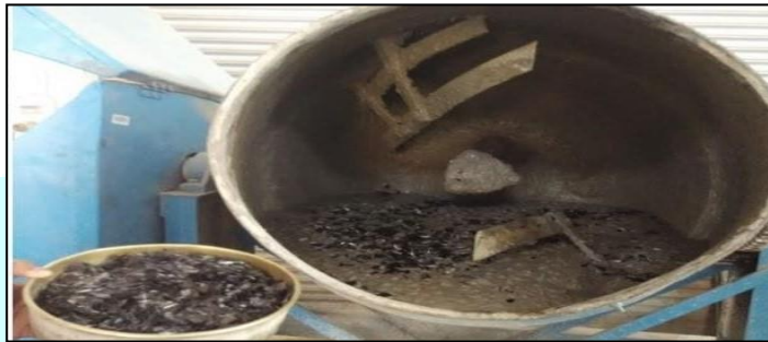
Fig. 3.3.1 Addition of Fiber to the SCC Mix
