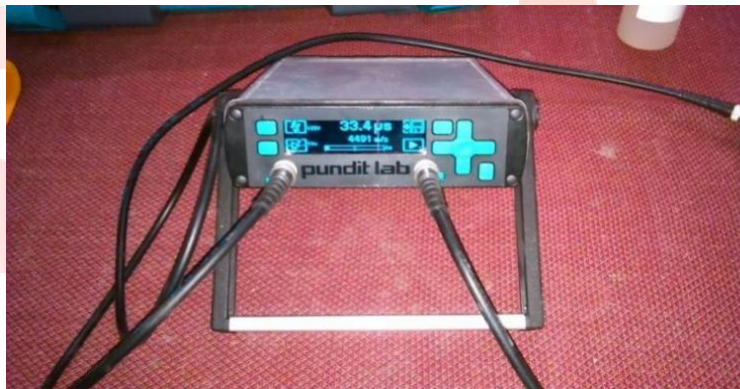
Fig. 3.4.1 UPV Test Set-up
