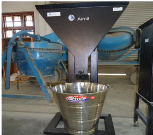
Fig.3.2.3.2 V-Funnel Apparatus & Schematic Diagram
