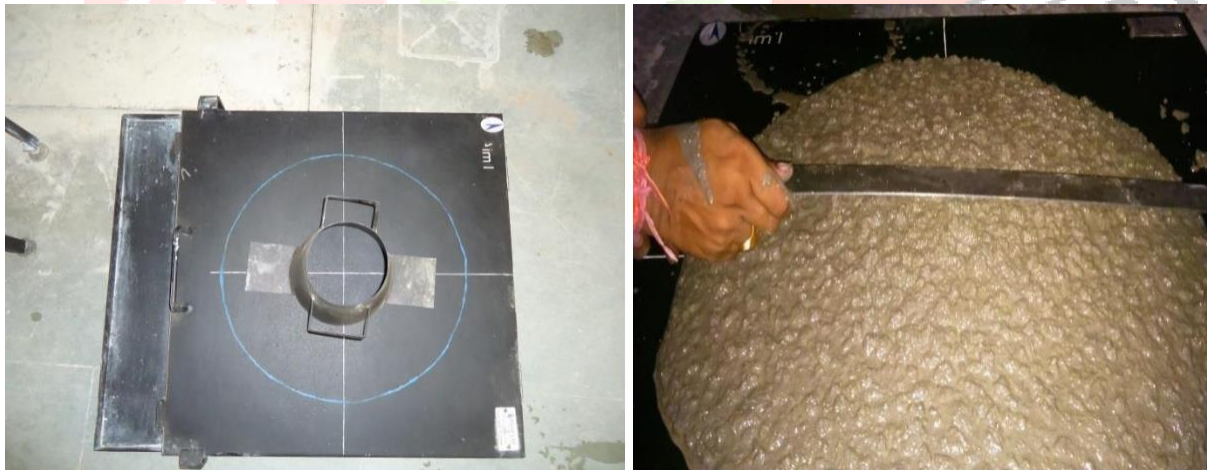
Fig. 3.2.3.1 Slump Flow Apparatus & Testing
