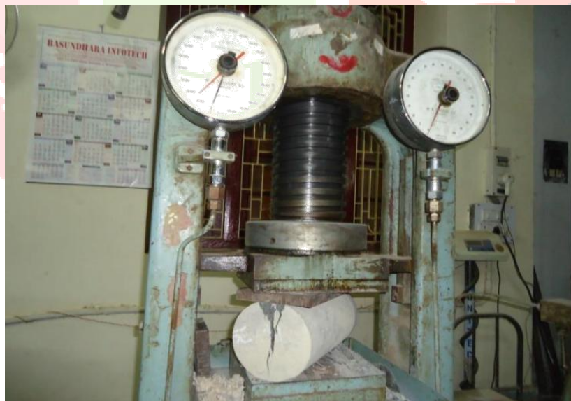
Fig: 3.2.6.2 Split tensile Test Set-Up
