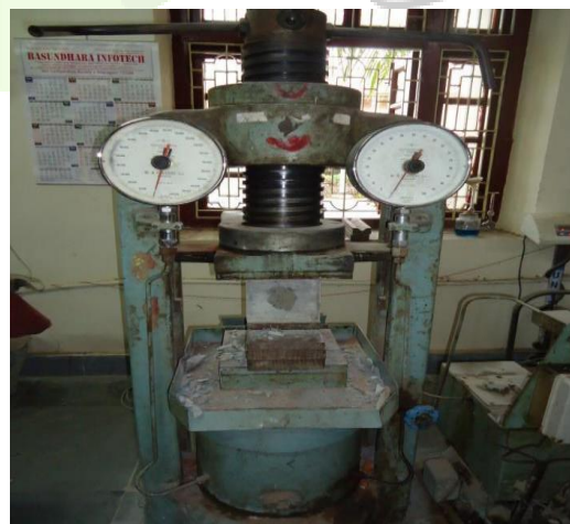
Fig: 3.2.6.1 Compression Test Set-Up
