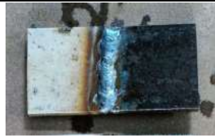
Fig.2 MIG Welded sample
