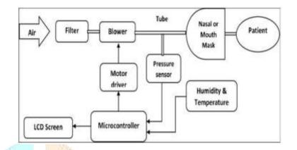
An artificial breathing machine with variable volume pressure and breath rate works by delivering a controlled amount of air to a patient's lungs. The machine is connected to the patient through a tube, which is inserted into the patient's airway.
