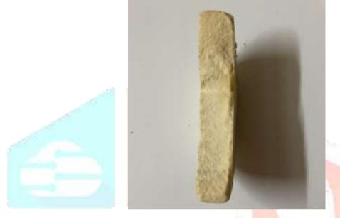
We used a saw to break the containers in half so that we could examine the contents because the soaps were difficult to remove from the containers due to their hardness.
