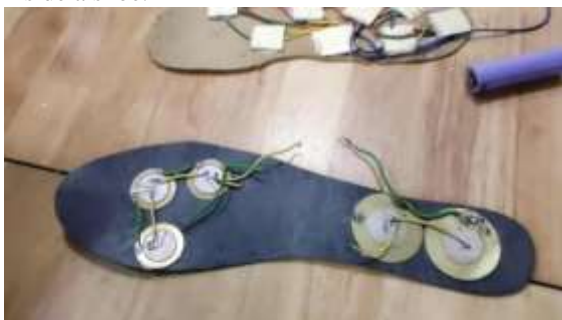
Fig:2. Arrangement of piezoelectric creator inside a shoe.
