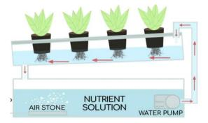
ii) Horizontal NFT System: In a horizontal NFT system, plants are grown in channels or gutters that are inclined slightly to allow the nutrient solution to flow continuously over the roots. The excess nutrient solution is collected at the end of the channel and returned to the reservoir for recirculation. This system is suitable for growing small plants like lettuce, herbs, and strawberries.
