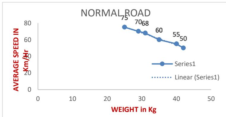
The average speed decreases with increase in weight. The load 75kg has maximum speed 19km/hr.
