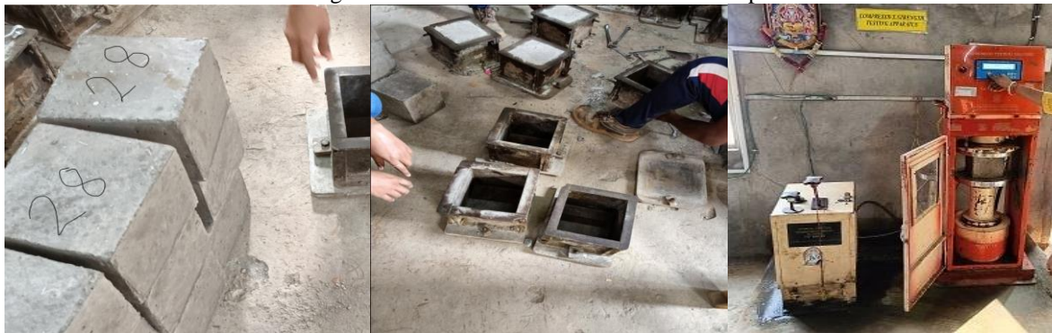
Fig no.-3.1 cement mortar with NS cube samples
