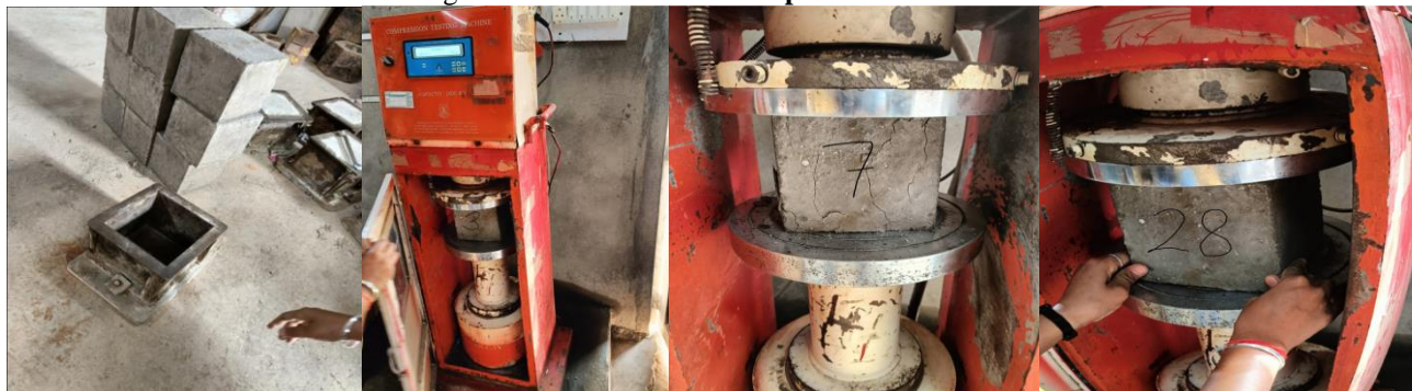
Fig no 3.2- concrete cube sample test
