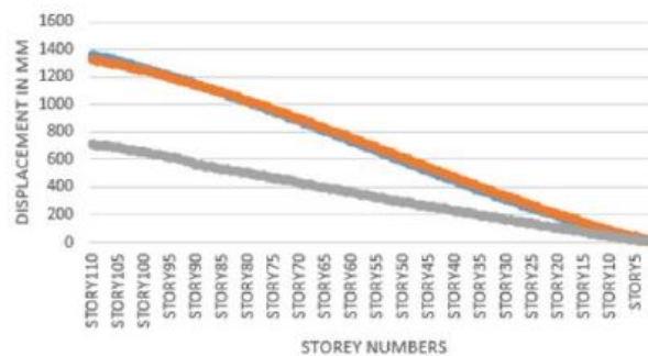
Fig 4.2: Displacement along soil type 2
