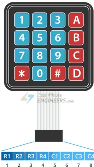
It is important to note that the pins used for the keypad can be changed in the code, but it is essential that the pins used for the rows and columns are connected to separate pins on the Arduino. This is because the rows and columns must be read and written to separately in order to detect key presses. In addition to its use as an input device, a 4x4 keypad can also be used for password authentication, security systems, or other applications that require user input.
