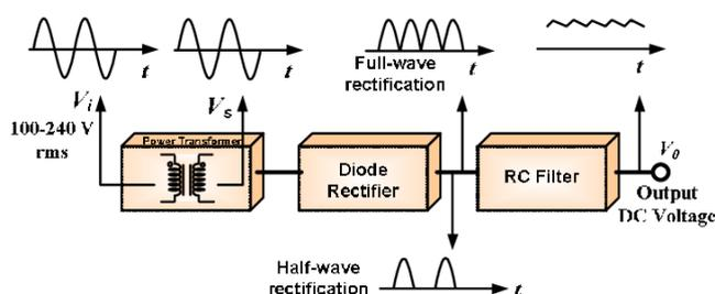
**Transformer:** The transformer is the first component in the power supply system. It takes in the 230V AC voltage input from the mains power source and steps it down to a lower AC voltage suitable for rectification. The transformer consists of two coils of wire wrapped around an iron core.
