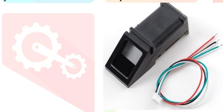
Once the R307 sensor is connected to the Arduino can start sending commands to the sensor to perform various operations such as fingerprint enrolment, fingerprint recognition, and template storage. The sensor has a simple and easy-to-use command set that can be accessed through the serial interface.
