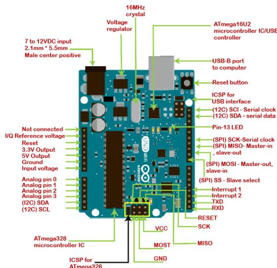
The board also has a power jack and an ICSP header for programming the microcontroller using an external programmer. The board is programmed using the Arduino Integrated Development Environment (IDE), which is a free software tool that provides a user-friendly interface for writing, compiling, and uploading code to the board. The IDE supports the C++ programming language and provides a large library of pre-written code, making it easy for beginners to get started with programming the board.
