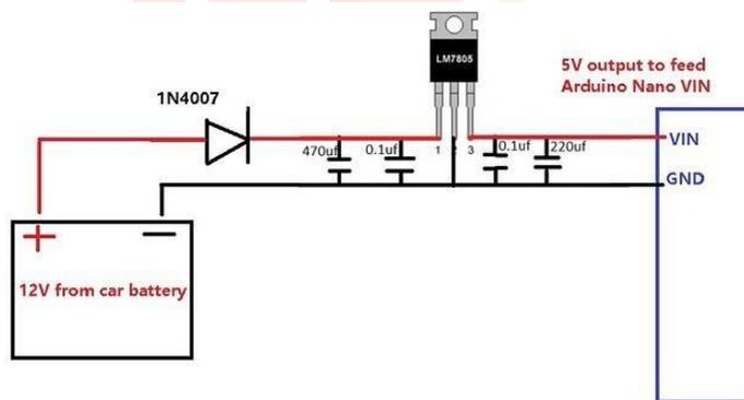
To use the converter, the positive and negative wires from the 12V battery are connected to the input terminals of the converter. The positive and negative wires from the output terminals of the converter are then connected to the device that requires 5V power. It is important to follow the
