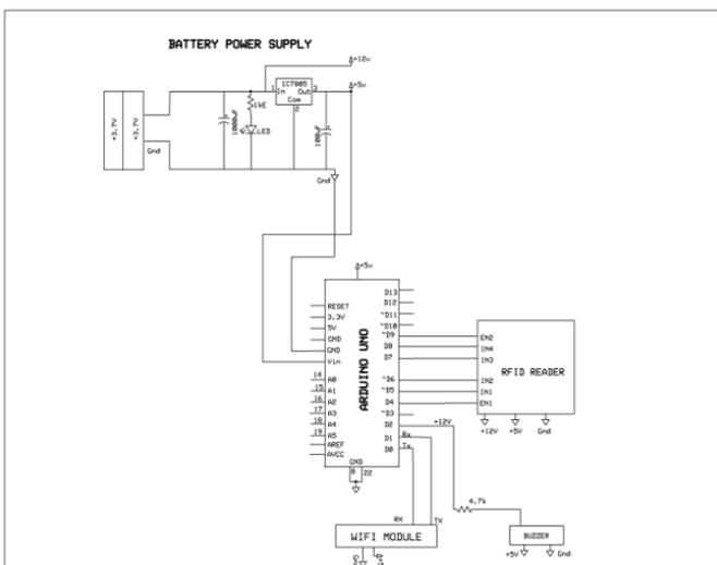
in its path. The NodeMCU will act as the main controller to collect data from all sensors and control the trolley's movement. The Arduino Uno will be used to control the four BO motors that drive the trolley. A WIFI module will be used to communicate with the trolley from a mobile application. A buzzer will provide audio feedback to the user, and an LCD will display the product information and billing details. The webserver will store all transactional data and generate bills automatically.
