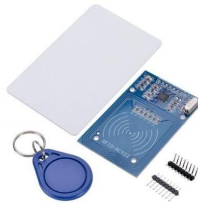
The RC522 RFID reader includes built-in security features, such as a 48-bit unique ID number for each device and support for encryption and authentication protocols. These features ensure the security and privacy of the data stored on the RFID tags and prevents unauthorized access to the system.
