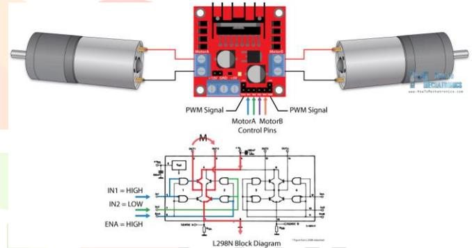
When using the L298N motor driver, it is important to follow the manufacturer's instructions and take necessary precautions to avoid electric shock or short circuits. Careful consideration of the motor specifications and control signals is also necessary to ensure proper operation and avoid damage to the motor or the IC.
