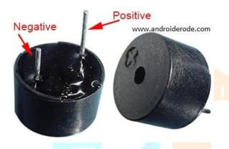
A buzzer, often known as a beeper, is a sound-producing signaling device. It might be mechanical, electromechanical, or piezoelectric in nature.
