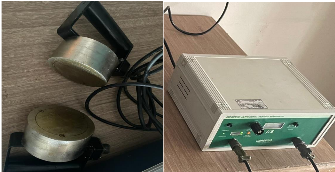
Figure 1 Transducer and Oscillatory signal measuring time
