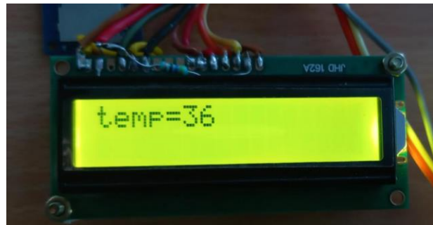
FIG: 5 TEMPERATURE VALUE DISPLAYED ON THE LCD DISPLAY
