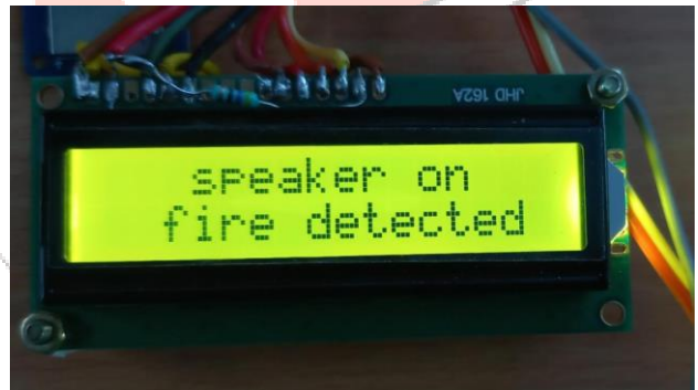
FIG: 6 FIRE DETECTED DISPLAYED ON LCD
