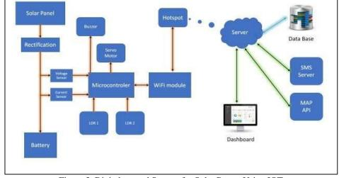
Figure 3. Digital control System for Solar Power Using IOT
