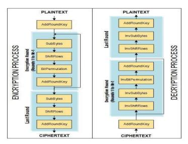
The algorithm is divided into four operational blocks where we observe the data at either bytes or bit levels and the algorithm is designed to treat any combination of data and is flexible for key size of 128 bits. These four operational blocks represent one round of Modified-AES. There are 10 rounds for full encryption. The four different stages that we use for Modified-AES Algorithm are:
