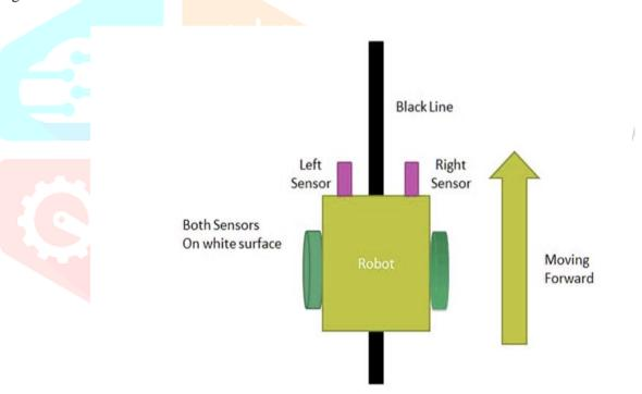
• The left sensor and right sensor IR sensor modules are used in this project. Robot advances when both left and right sensors detect white.
