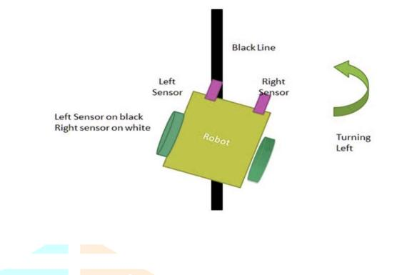
• If the right sensor detects a black line, the robot will turn right until the white surface is reached by both sensors. Robot resumes forward movement as soon as a white surface appears.
