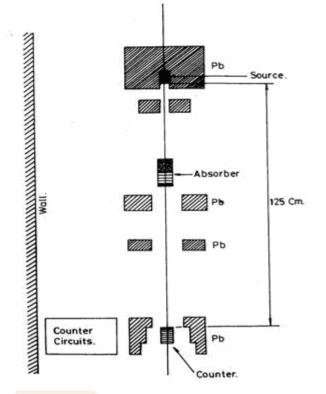
Fig. 1 The schematic view of the experimental set up.
