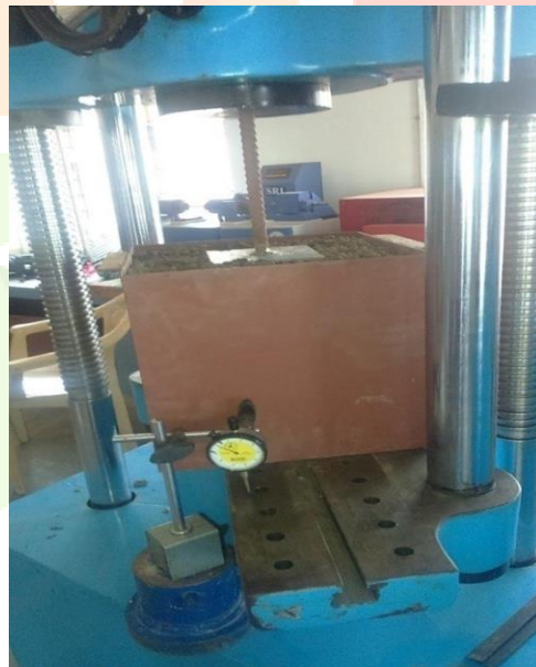
Fig 3.2 : Test Arrangement using UTM
