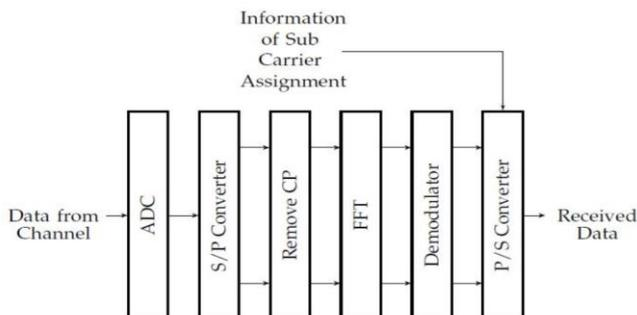
Figure 2: OFDM Receiver Block Diagram
