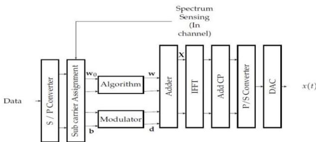
Figure 1: OFDM transmitter block Diagram
