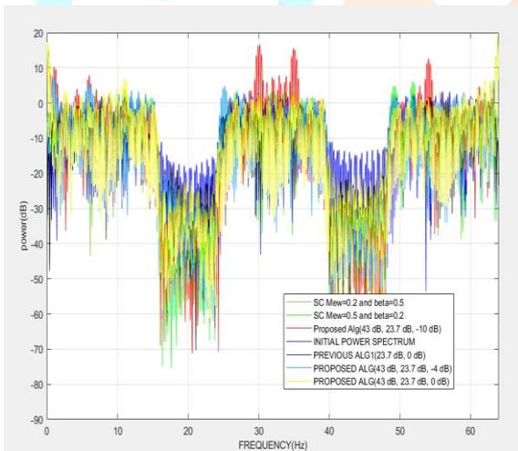
Figure 4: Power Spectral density of NC-OFDM for various algorithms
