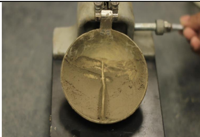
Figure 2.4 LL test on admixed BC soil specimen
