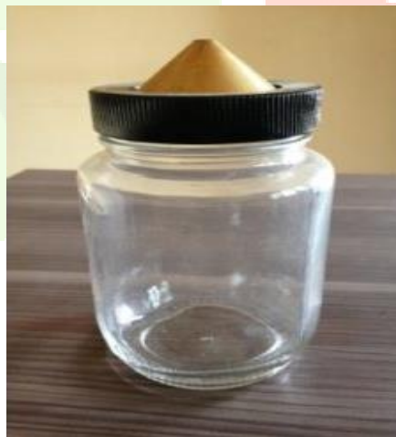
Figure 2.3 Pycnometer Used For Specific Gravity Test
