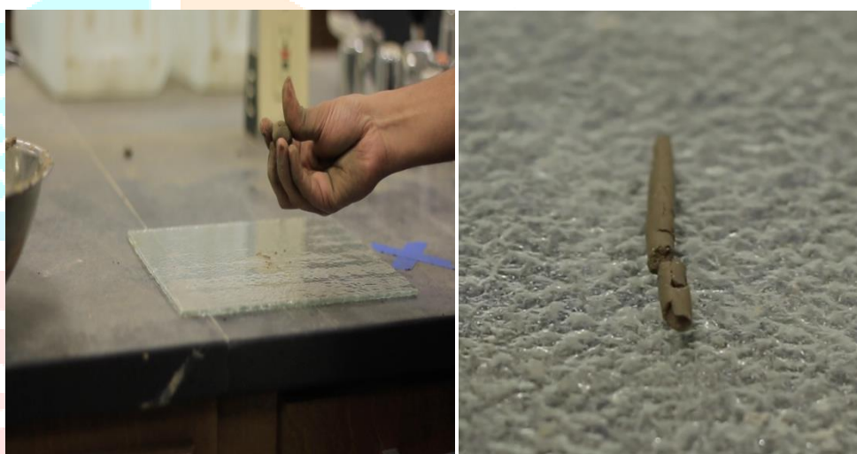
Figure 2.5 PL test on admixed soil specimen
